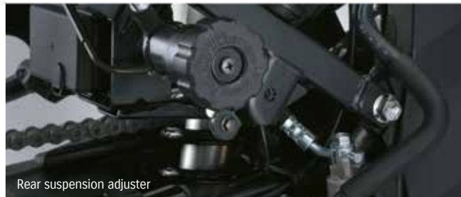
Rear suspension adjuster
