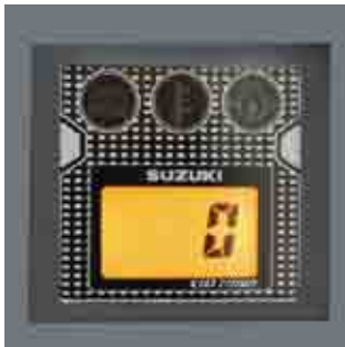
Tachometer with warning indicators
