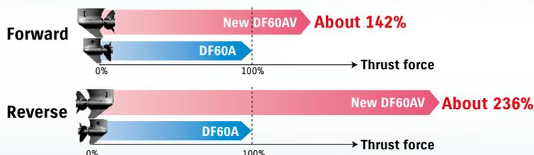
\* Thrust was statically measured using a stationary test boat running forward at 3,500rpm and reverse at 3,200rpm.
