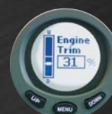
Engine trim page as a trim gage for single engine
